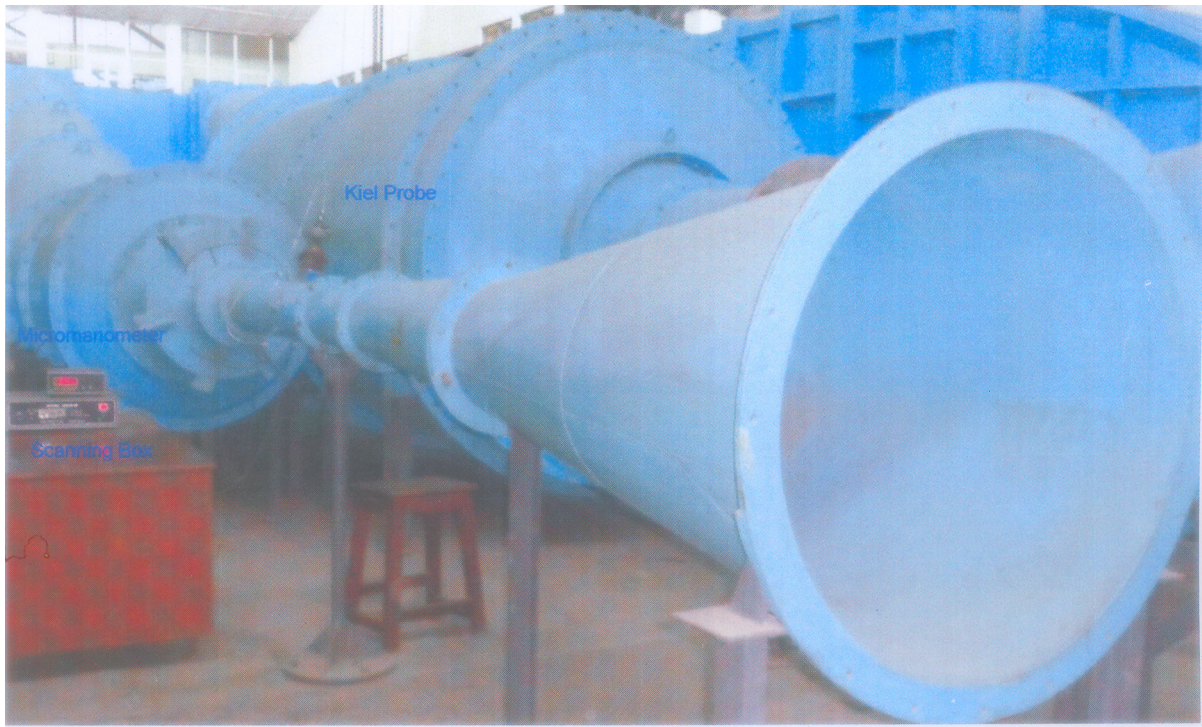
Fig.3 Calibration Tunnel, Calibration Device, Instrumentation and Probe
