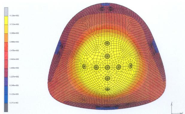
Fig.5 Temperature Profile for Max. Temperature Load Case (299s) Max. Temperature = 442°C (Figure shown ΔT only)
