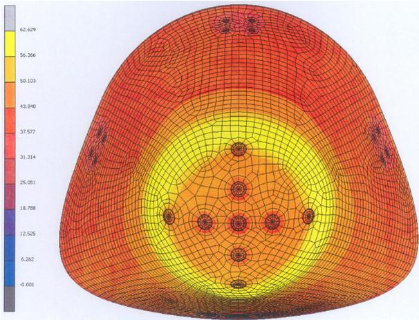
Fig.6 Temperature Profile for Max. Pressure Load Case (61s)
