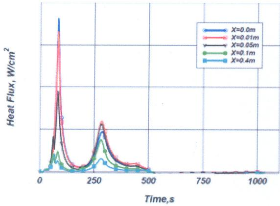
Fig.10 Predicted Heat Flux History of RLV C-C Nosecap
