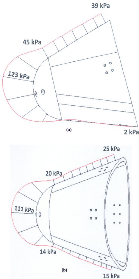
Fig.7 Pressure Profile on Nosecap for Max. Dynamic Pressure Loadcase (a) Side View (b) Top View
