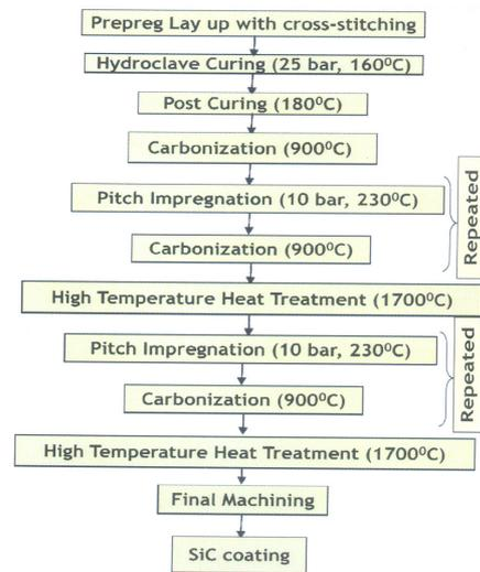
Fig.8 Generalized Process Route for C-C Nosecap
