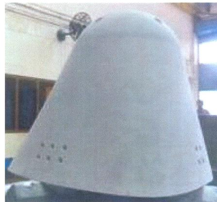
Fig.13 Carbon Nosecap with SiC Coating Ready for Assembly to RLV-TD Fuselage
