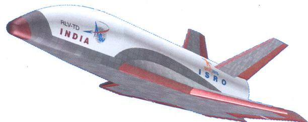
Fig.1 Reusable Launch Vehicle - Technology Demonstrator
