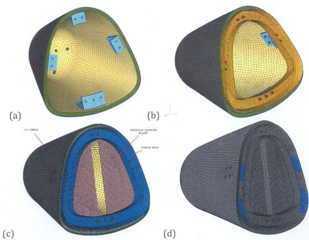
Fig.3(a,b,c) Finite Element Model of Nosecap (d) Fixity Locations for Nosecap Assembly at FNB Ring (in Blue)
