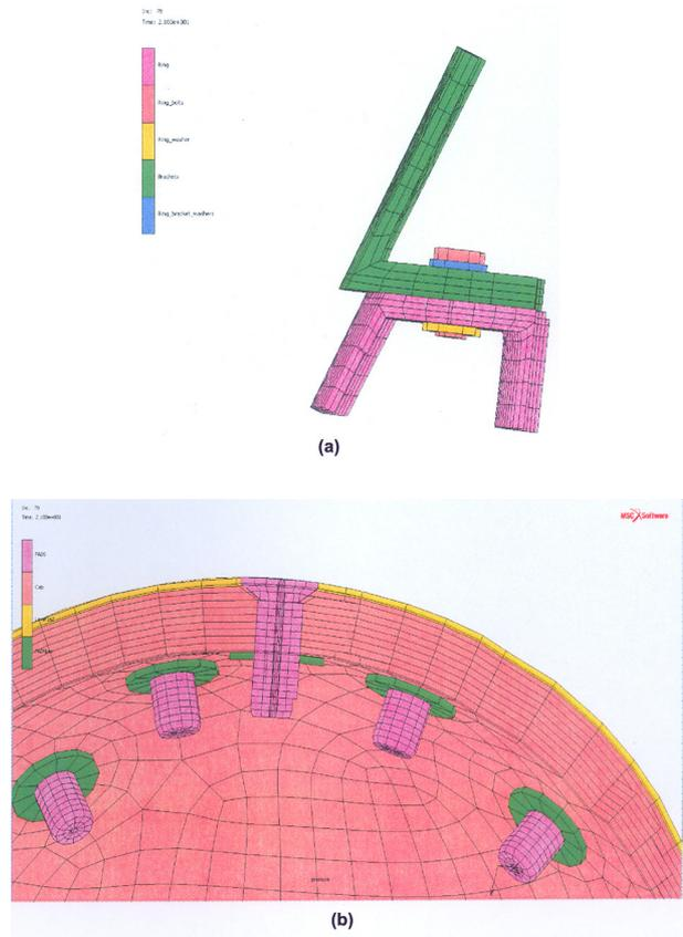
Fig.4(a) Section of FNB Ring and Clamp Joint
