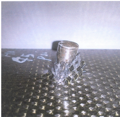
Fig.4 Embedded Condition of Bullet for 140 °C Loading Sample
