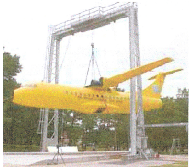
Fig.12 Drop Test on a Full Scale Commuter Aircraft
