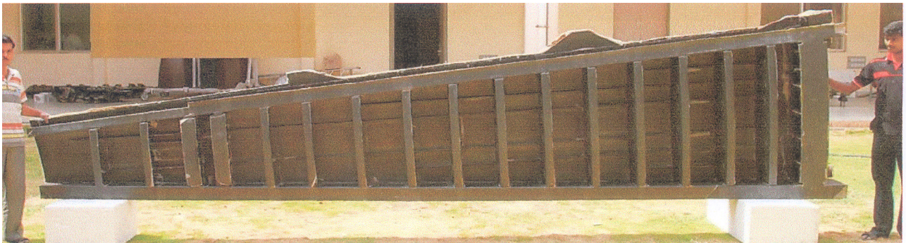
Fig.16 Resin Infused Wing Skin with Spars, Ribs, Stringers and Gussets for CSIR-NAL's SARAS Aircraft
