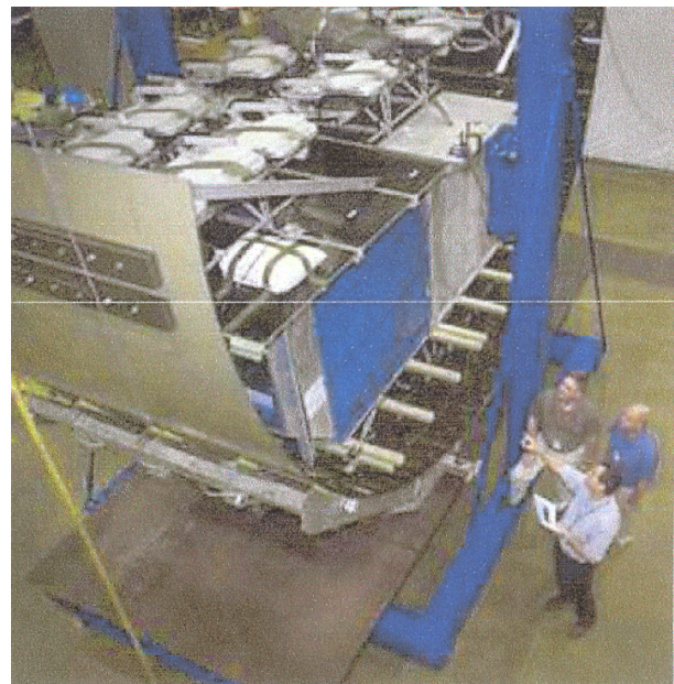
Fig.13 Drop Tests being Conducted on a Boeing 787 Fuselage
