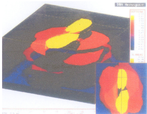
Fig.1 Time of Flight Ultrasonic C-scan Image of Impact Damage in a Quasi-Isotropic Carbon Fiber-Epoxy Laminate
