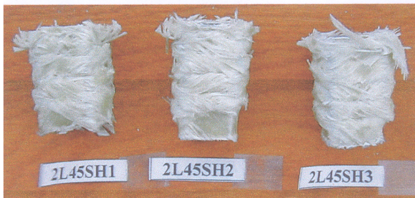
Fig.5 Folding pattern of square hybrid tubes with two layers of \pm 45^\circ E-glass/epoxy overwrap on a 25mm x 25 mm x 1.6 mm square aluminum (6063-T52) tube (from Ref.11)
