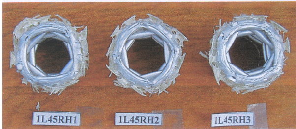
Fig.4 Folding pattern of round hybrid tubes with one layer of \pm 45^\circ E-glass/epoxy overwrap on a 50-mm diameter, 1.24 mm thick round aluminum (6061-T6) tube (from Ref.11)
