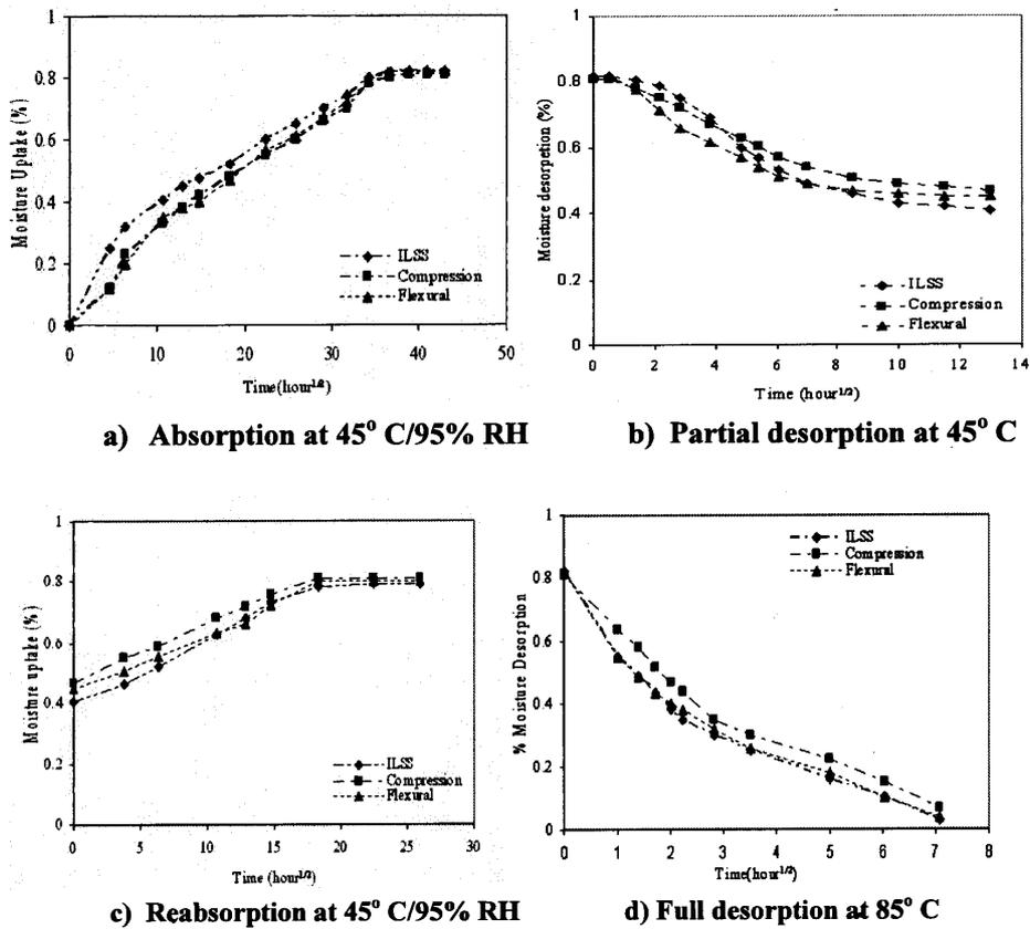
Fig.1 Moisture Absorption and Desorption Curves
