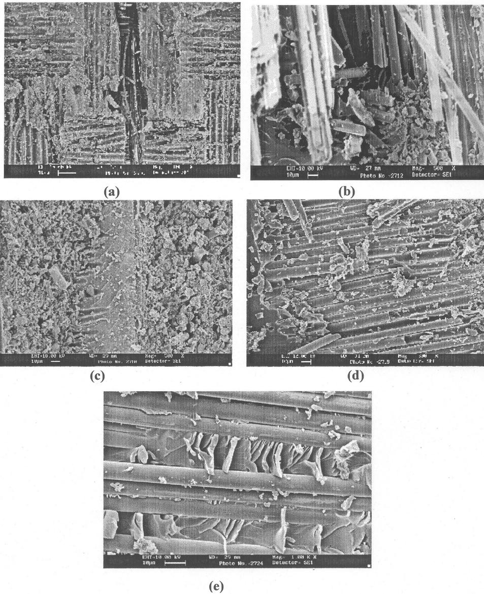
Fig.5 SEM Micrographs of the Fracture Surface of (a) - (b) dry and (c) - (e) aged Specimens
