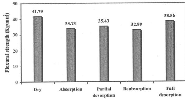
Fig.4 Flexural Strength of Glass-epoxy Composite
