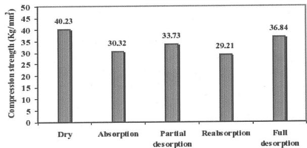
Fig.3 Compression Strength of Glass-epoxy Composite
