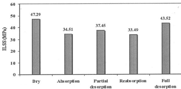
Fig.2 Interlaminar Shear Strength of Glass-epoxy Composite
