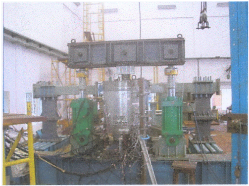
Fig.7 Loading Testing of 21 Turb Armature Coil Assembly
