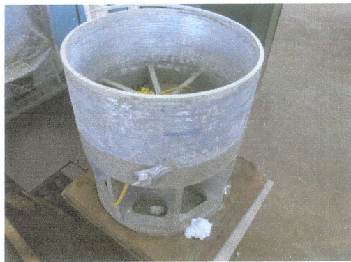
Fig.8 Armature, After Tension Bonding
