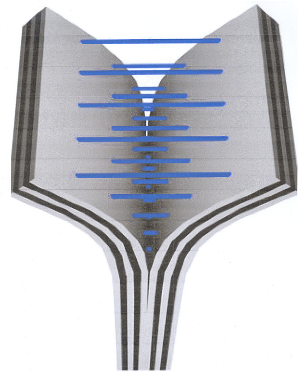
Fig.9 Carbon Fiber Reinforced Polymeric Composite Plies Stitched Together with CNTs [Ref.29, 30]
