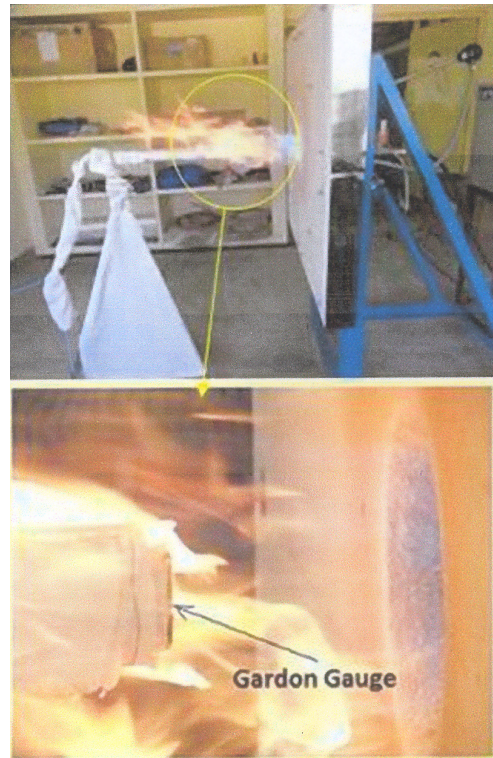
Fig.2 Photographic Views of Gardon Gauge Heat Flux Sensor in Plume
