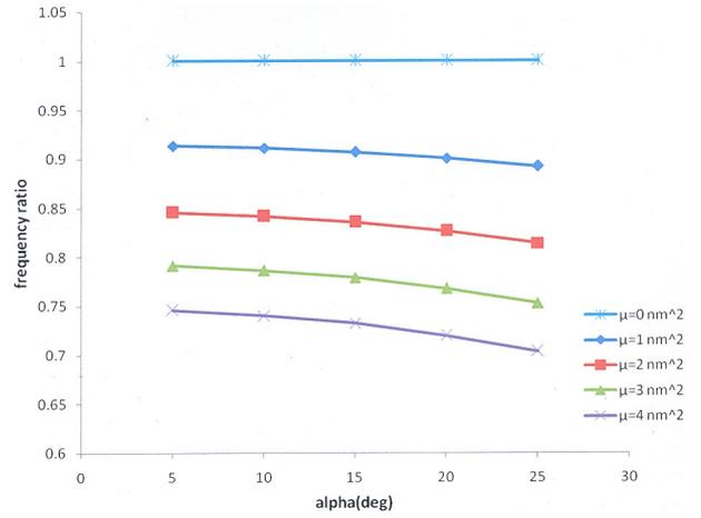
Fig.5 Frequency Ratio Vs  $\alpha$  (deg) for  $m=n=1$ ,  $L = 10 \text{ nm}$  and Various Nonlocal Parameters
