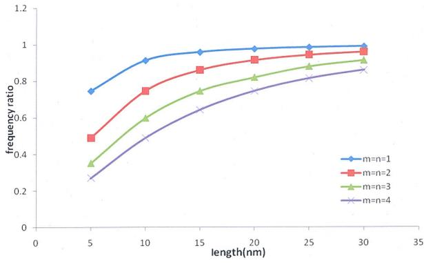
Fig.4 Frequency Ratio Vs Length for  $\alpha = 5 \text{ deg}$ ,  $\mu = 1 \text{ nm}^2$  and  $m = n$
