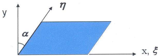
Fig.1 Skew Graphene Sheet with Co-ordinate Axis
