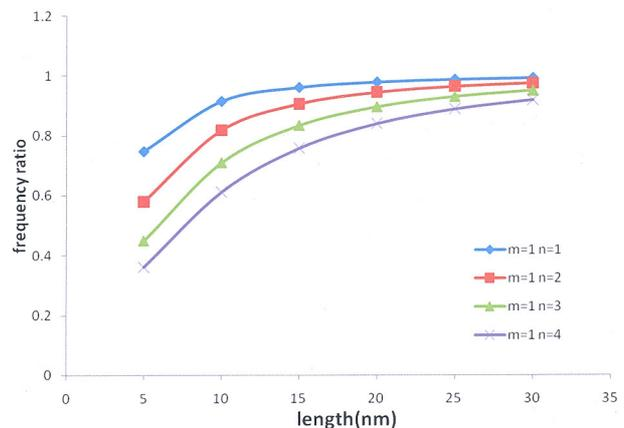
Fig.3 Frequency Ratio Vs Length for  $\alpha = 5 \text{ deg}$ ,  $\mu = 1 \text{ nm}^2$  and  $m \neq n$
