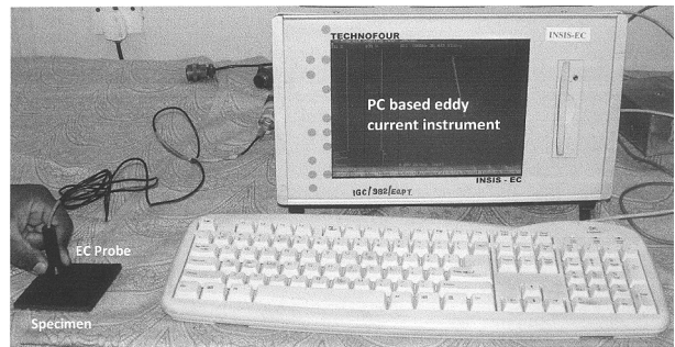
Fig.2 Eddy Current Test Set-up Used for Assessment of Thickness of SiC Coating on C/C Composite Specimens
