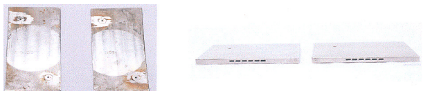
Fig.12b Bond Strength Specimen Brazed, Pressure Tested and Sectioned
