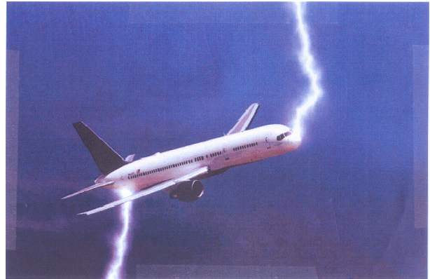
Fig.5 Lightning Entering and Exiting from a Plane [10]
