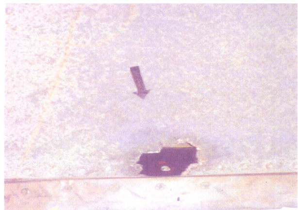
Fig.1 Hole Burned Through the Top of Wing in 1963 PAN AM Boeing 707 (Atmospheric Science University at Albany)
