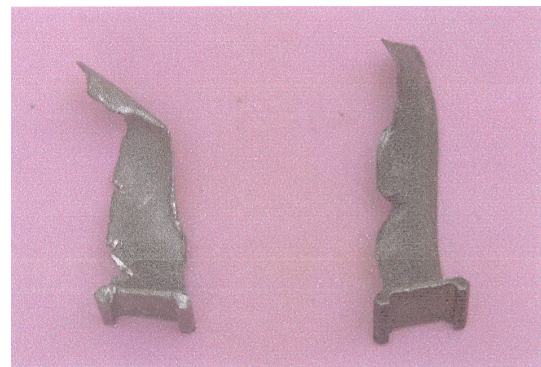
Fig.8 State of the Stator Vanes Due to Surge
