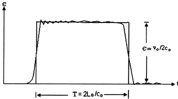
Fig.5 Schematic of pressure pulse in incident bar
