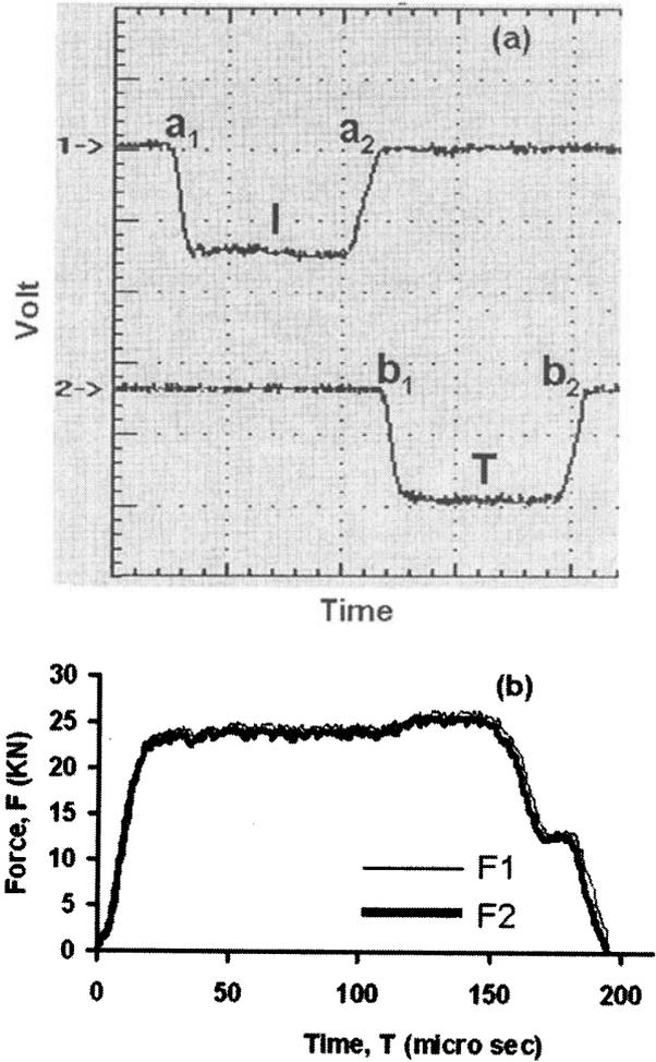
Fig.4 Compressive SHPB test results obtained during calibration : (a) strain gauge signals on oscilloscope, (b) comparison of force versus time behaviour, derived from strain gauge signals
