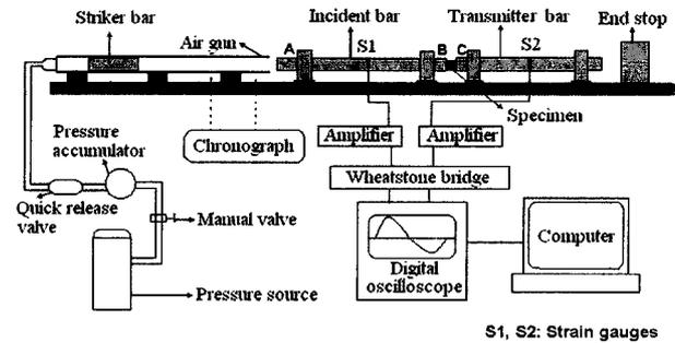
Fig.2 Schematic of compressive Split Hopkinson Pressure Bar apparatus
