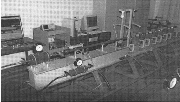
Fig.3 Photograph of compressive SHPB apparatus
