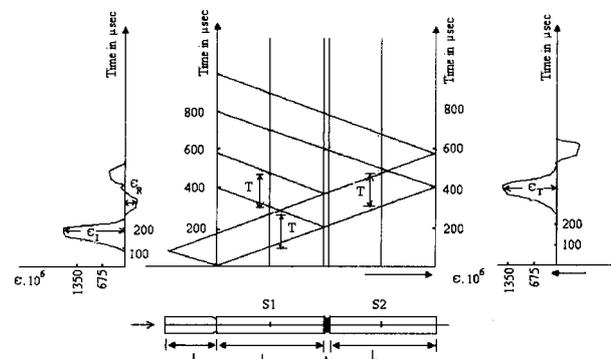
Fig.1 Stress wave propagation in Split Hopkinson Pressure Bar
