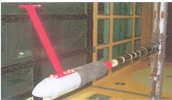
Fig.8b Adapter Mounted on the Load Balance
