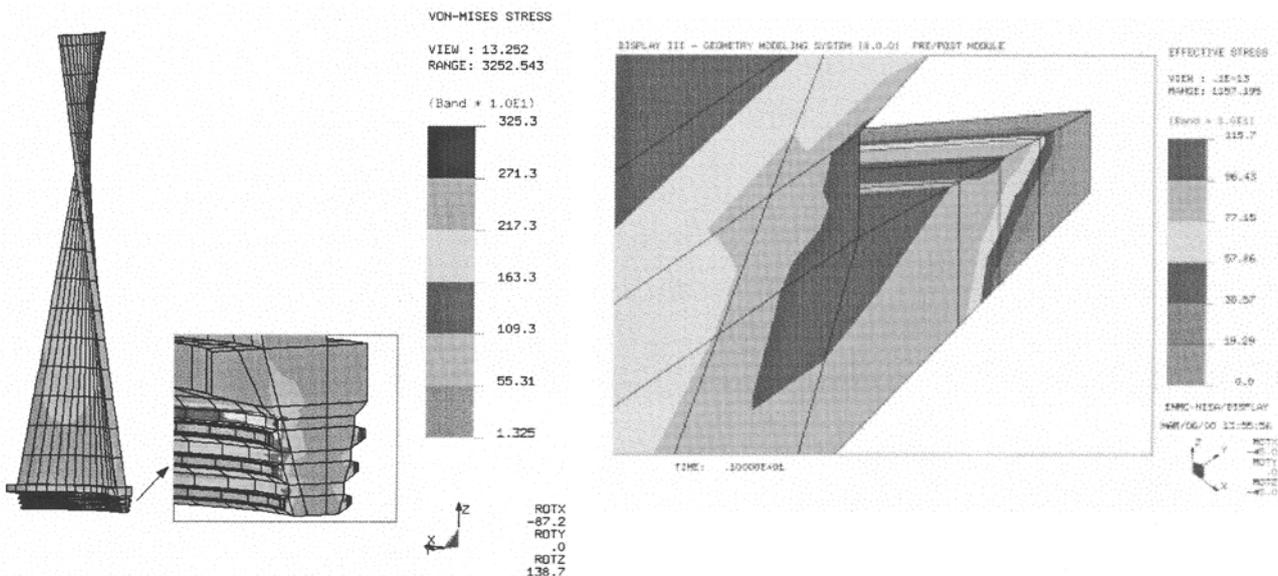
Fig.11 Elastic and elasto-plastic analysis of a last stage steam turbine blade
