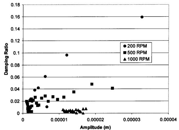
Fig.13 Analytically estimated damping in a rotating bladed-disk due to combined friction and material deformation at slipping surfaces
