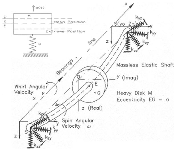
Fig.1 Jeffcott rotor model on 8 coefficient bearings
