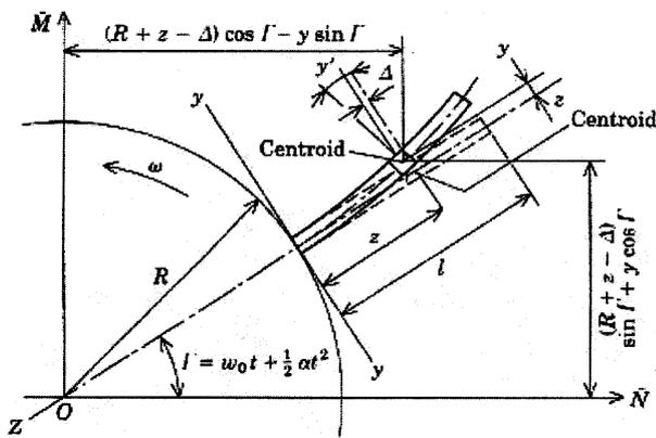
Fig.14 Rotating blade modeled as a beam
