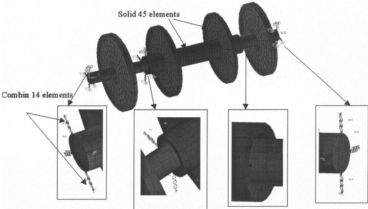
Fig.6 Full solid rotor model
