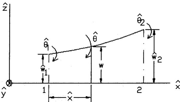
Fig.3b Shaft element in  $xz$  plane
