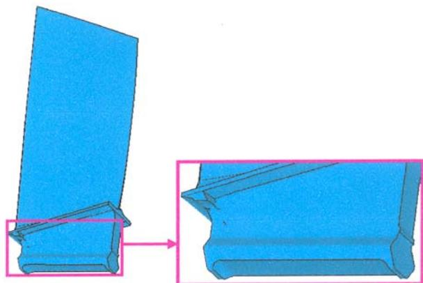
Fig.17 A compressor blade root for weight optimization
