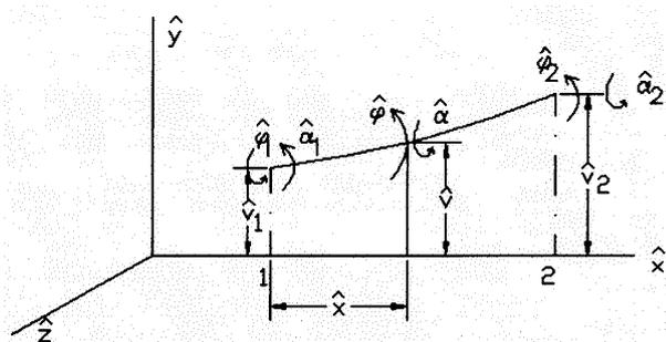
Fig.3a Shaft element in  $xy$  plane
