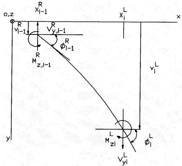
Fig.2c State quantities for transfer matrices in plane xy
