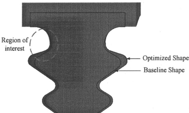
Fig.16 Blade root shape optimization
