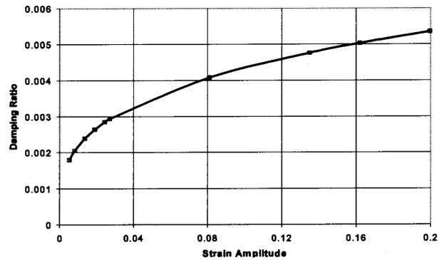
Fig.12 Analytically estimated material damping
