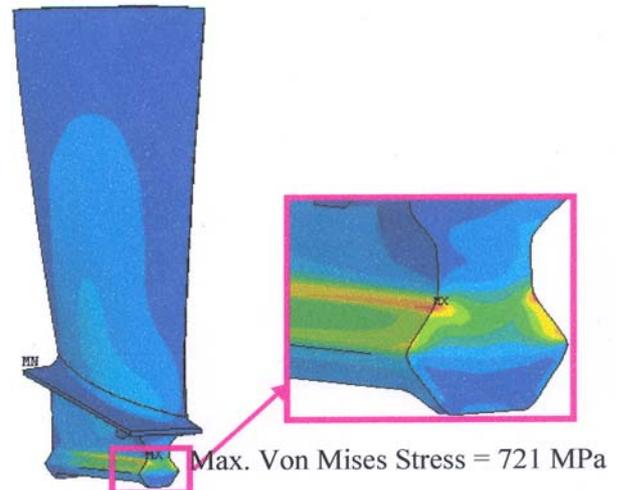
Fig.18 Baseline stress result under centrifugal loading
