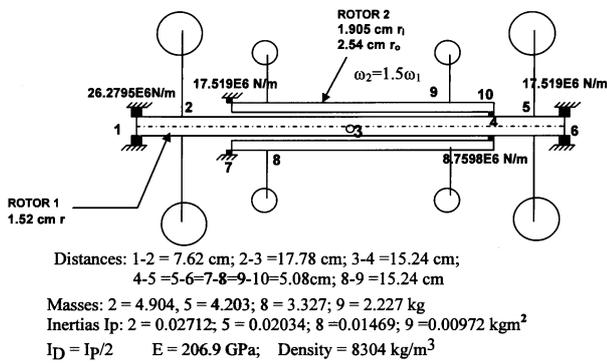
Fig.4 Example of a twin spool rotor
