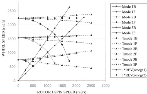
Fig.7 Campbell diagram of twin spool rotor system
