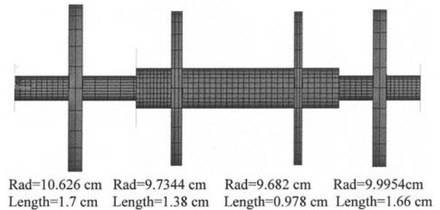
Fig.5 A solid rotor model of Fig.4
