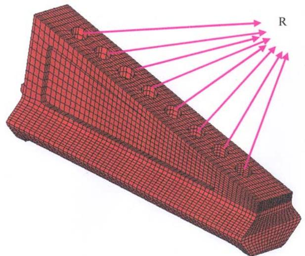
Fig.19 Blade shank baseline generated for optimization with 8 holes and two cutouts in the shank
