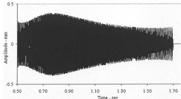
Fig.10 Coast up response of a high speed turbo pump with acceleration 1800 rad/sec2
