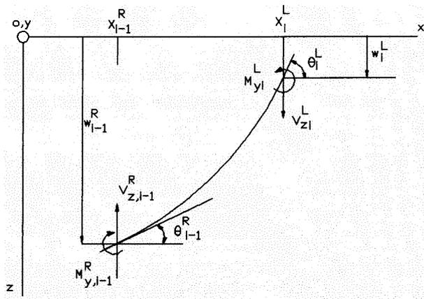
Fig.2b State quantities for transfer matrices in plane xz
