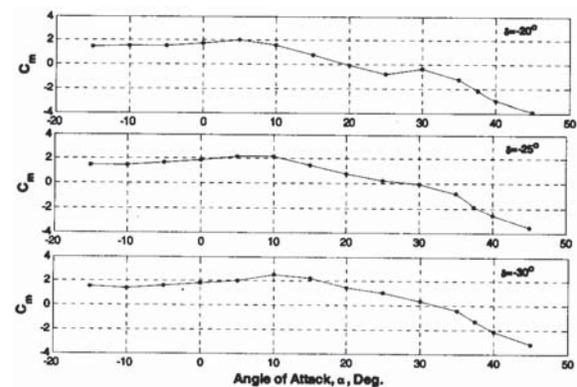
Fig. 4 Pitching moment coefficient Vs. angle of attack for body with fin at  $\delta = -20^\circ, -25^\circ, -30^\circ$
