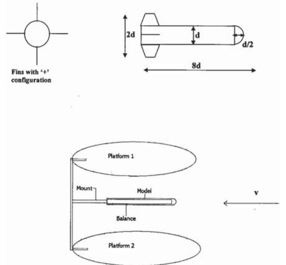
Fig. 1 Schematic of the model and the fitment used in wind tunnel testing
