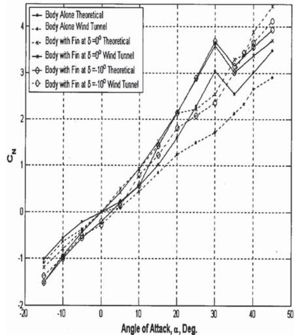
Fig. 2 Comparison of wind tunnel theoretical estimates of normal force coefficient for body alone and body with Fin at  $\delta = 0^\circ, -10^\circ$
