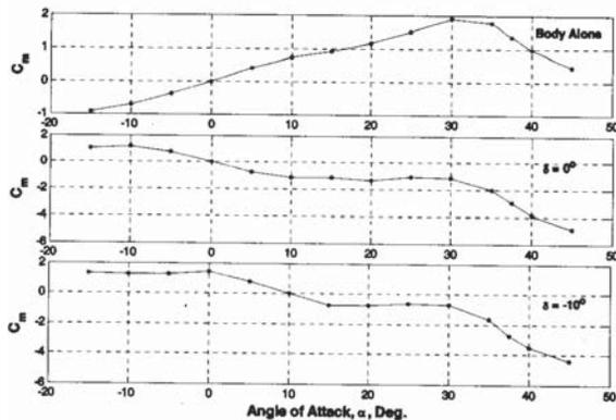
Fig. 3 Pitching moment coefficient Vs. angle of attack for body alone and body with fin at  $\delta = 0^\circ, -10^\circ$
