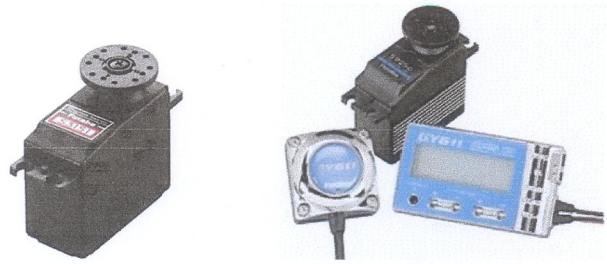
Fig.9 Futaba S3151 Servo (Left) and S9256 Servo with GY611 Gyro and Controller (Right)
