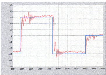
Fig.31 Closed Loop Yaw Angle Control for Set Points +30 deg and -30 deg
