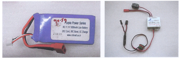
Fig.17 LiPo Battery - 11.1 v at 1000mAh Capacity and an 8A UBEC
