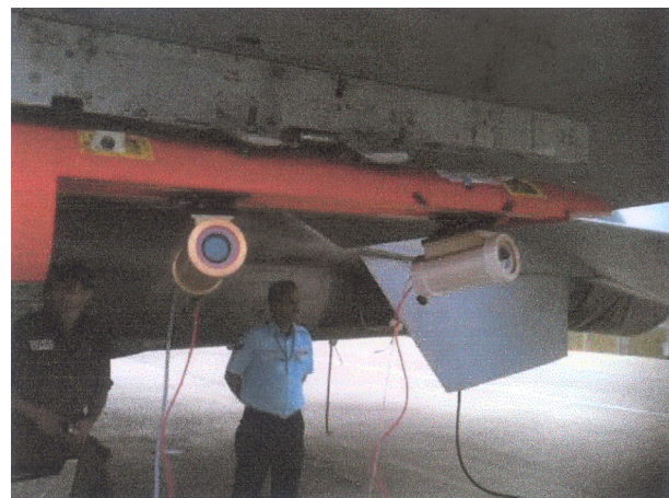
Fig.1 Two High Speed Cameras Looking Towards Outer Station on Su 30MK1
