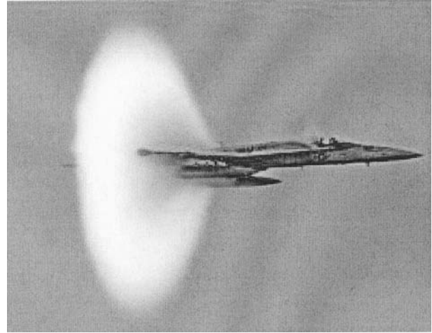
Fig.4 F-18A condensation cloud near M = 1
