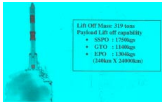
Fig.2 PSLV-XL and its payload capability
