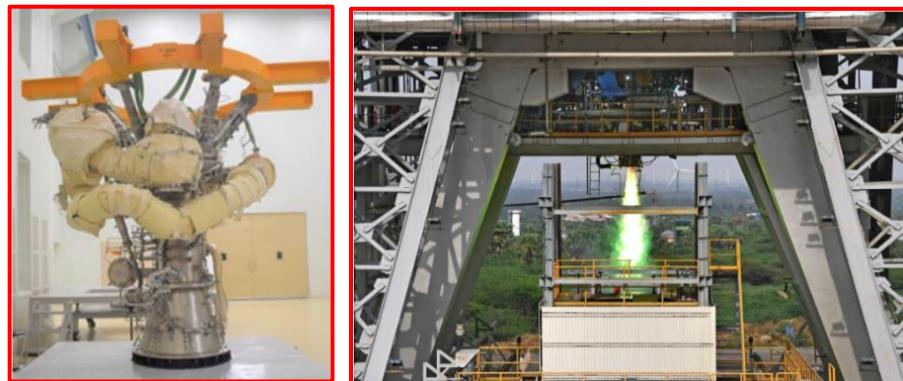
Pre-Burner Ignition Test Article and Hot test being performed
