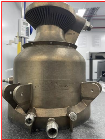
3D printed Single Piece Rocket Engine
