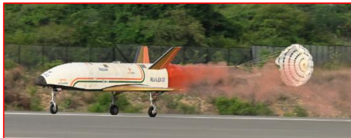
Reusable Launch Vehicle (RLV) Landing EXperiment (LEX)
